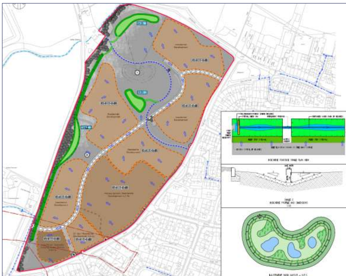
Figure 4-3: Extract from illustrative drainage strategy WSP drawing ref 4147-D-02
