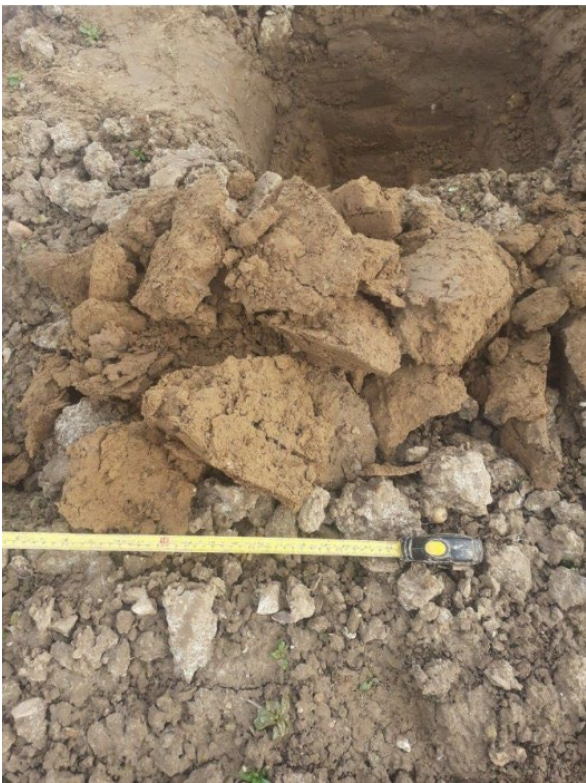
Upper subsoil as excavated
