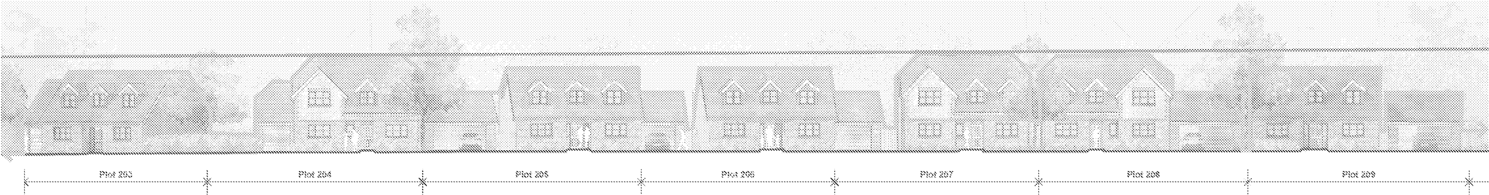
Roof Line of New Street Scene M-M CA4a - Greater variation in roof height, maximum roof height indicated in blue.
