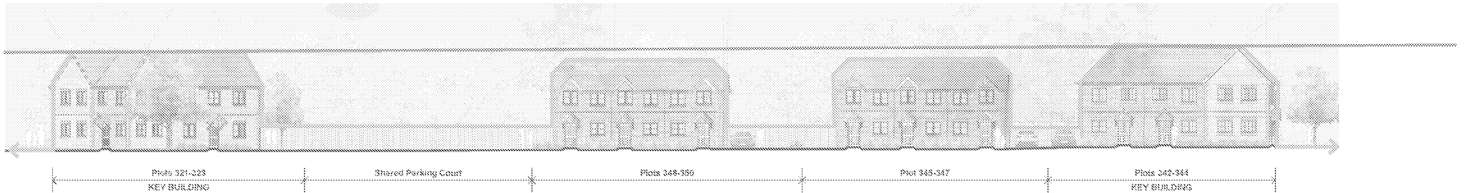
Roof Line of New Street Scene P-P CA4a - Greater variation in roof height, buildings reoriented and reposition to increase active frontage, maximum roof height indicated in blue.
