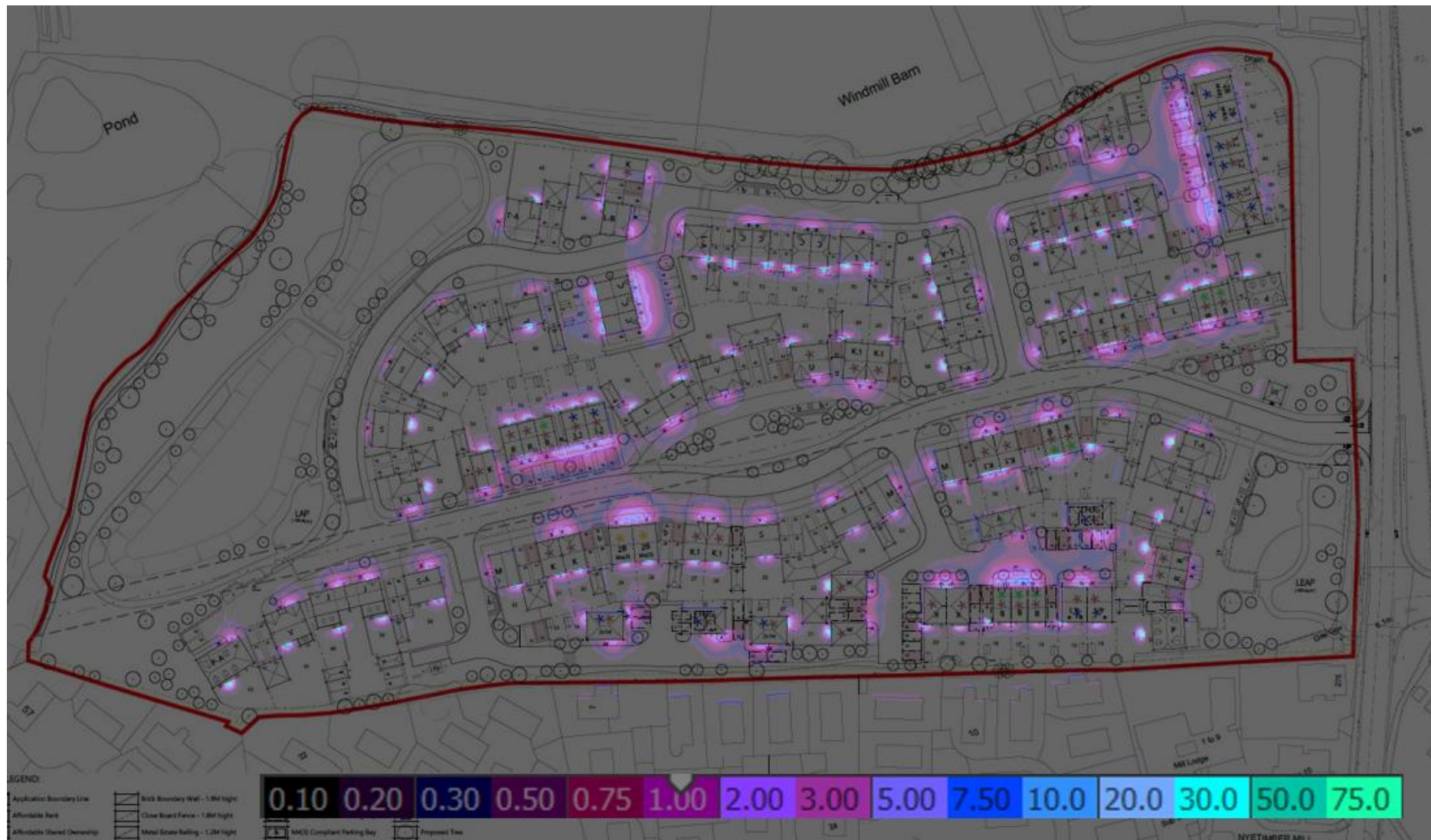
Figure 5-3 - Visual Representations of Lux Contour Plot
