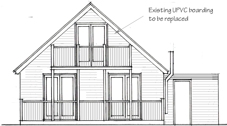
SOUTH ELEVATION (REAR)
