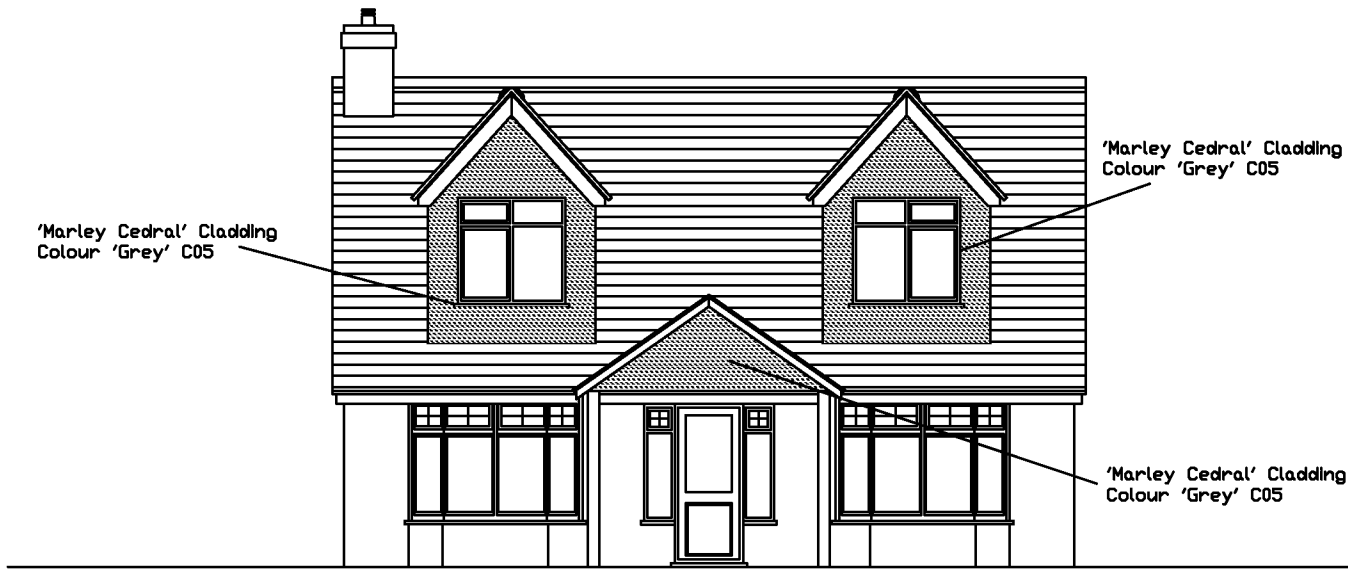
Proposed North W/West Elevation
