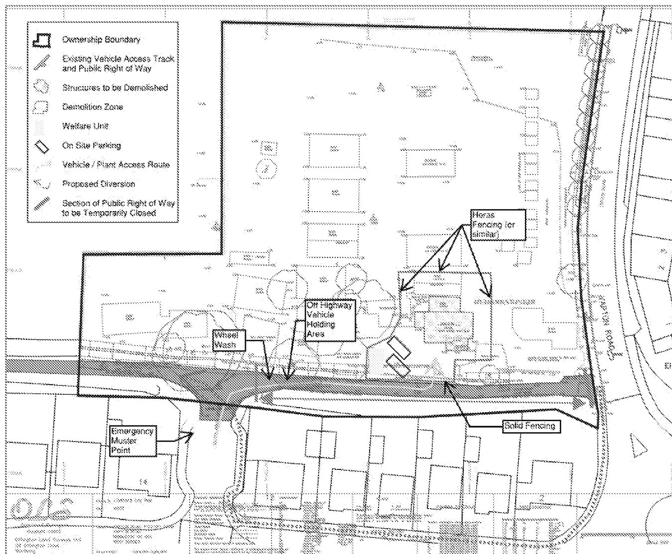
Figure 5-2: Schematic of Site Layout During Demolition (Phase 1)
