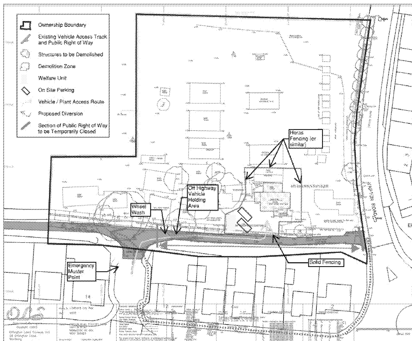
Figure 5-2: Schematic of Site Layout During Demolition (Phase 1)
