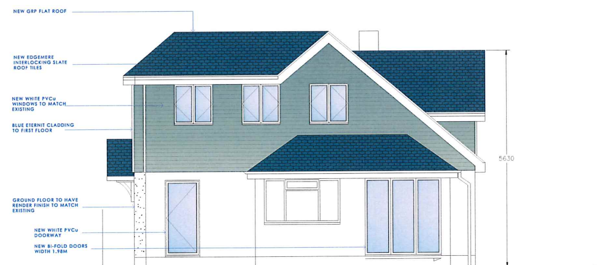
ELEVATION FACING SOUTH
