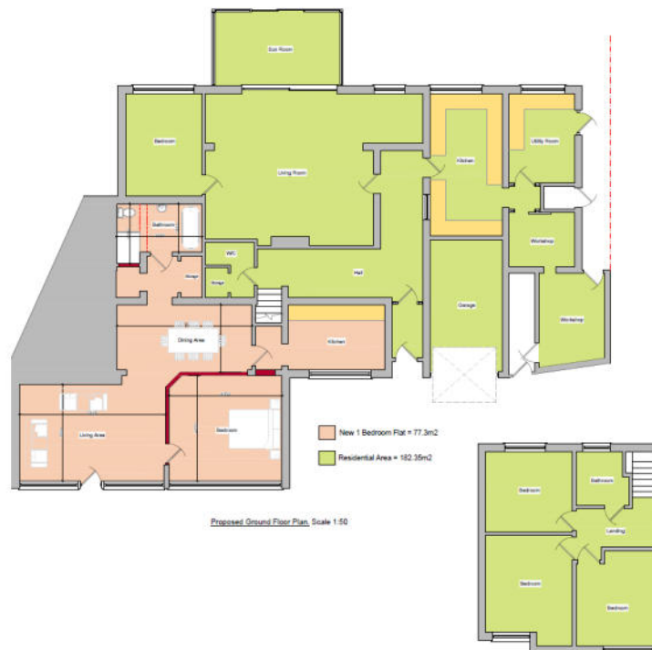
Fig 8. Proposed Ground Floor Plan and First Floor Plan (affected site area shaded peach)
