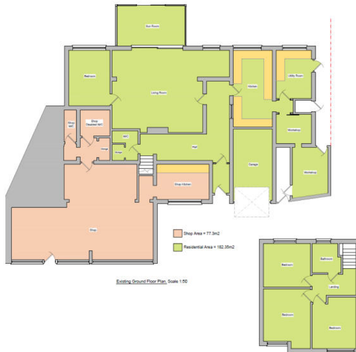
Fig 7. Existing Ground Floor Plan and First Floor Plan (affected site area shaded peach)
