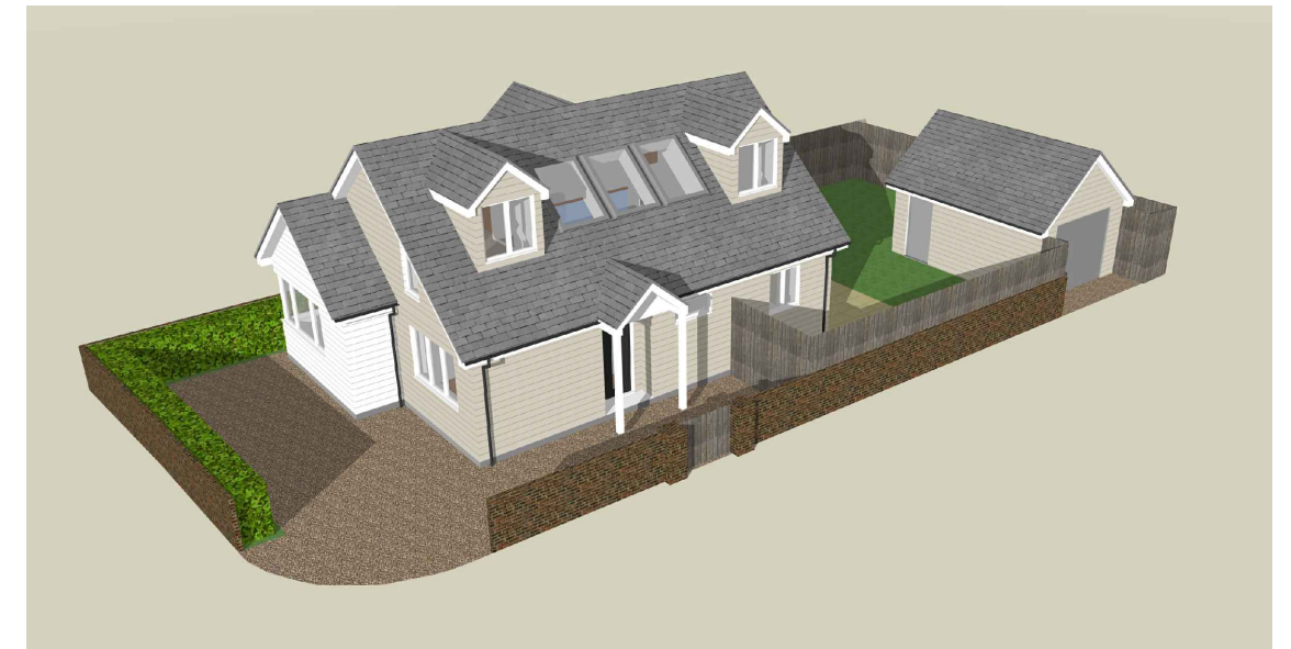
aerial view of house as proposed with new dormers, skylights, roofing and cladding
