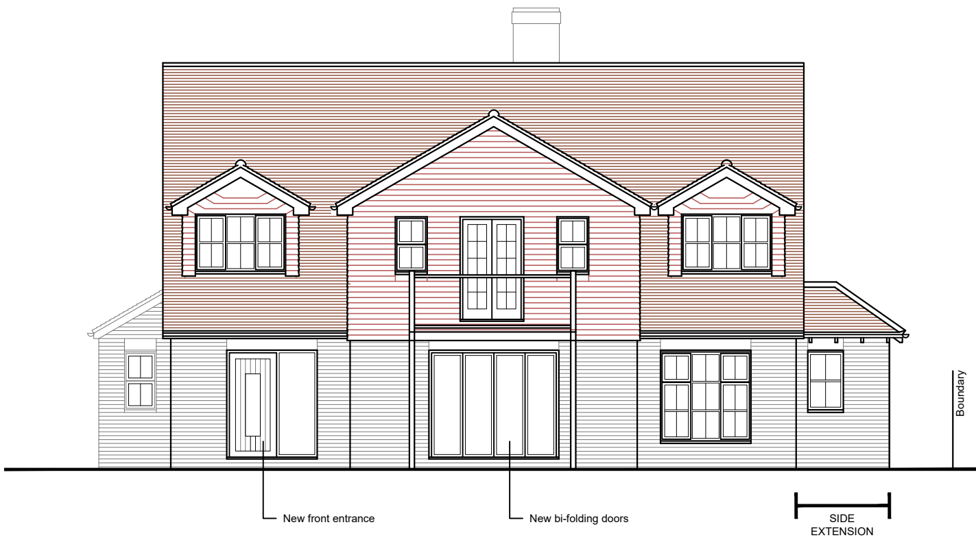
FRONT ELEVATION [west] 1:100
