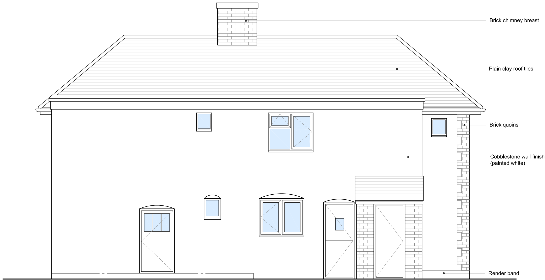
EXISTING REAR ELEVATION 1:50
