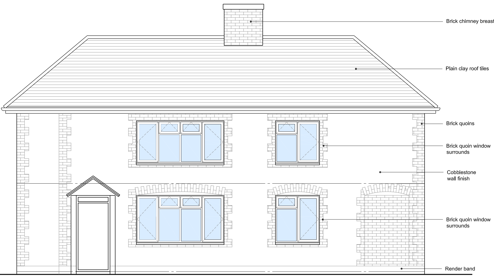
EXISTING FRONT ELEVATION 1:50
