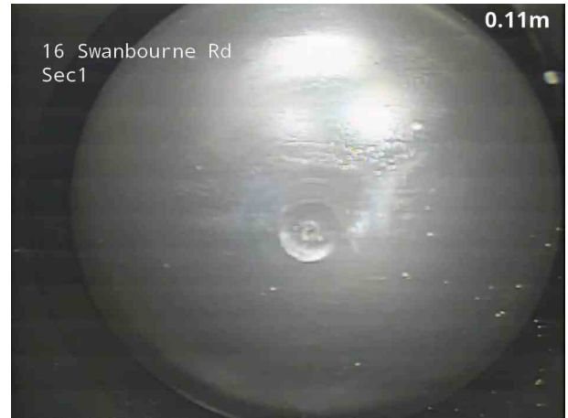
2, 00:00:31, 0.10 m Finish node, manhole, reference: A. Capped
