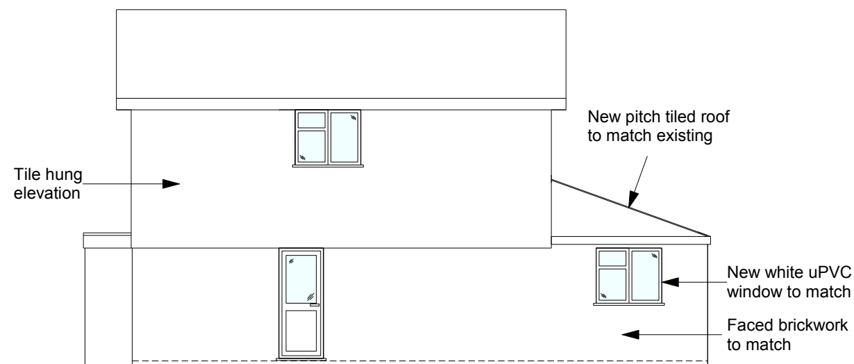
Side Elevation Proposed (South) Scale 1:100
