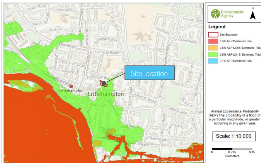
Figure 5.6: Modelled Flood Outlines Undefended (Tidal)
