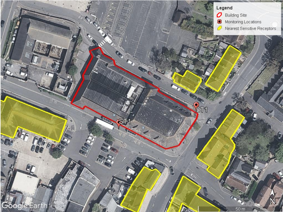
Figure 3-1: Satellite image showing noise measurement locations and nearest noise sensitive receptors (courtesy of Google)
