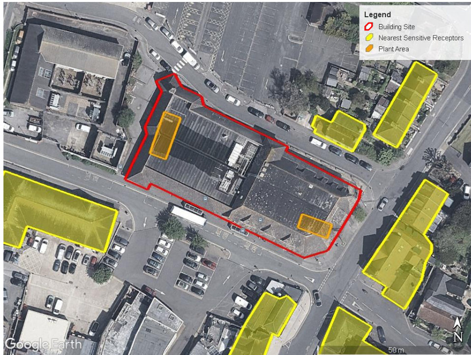
Figure 4-2: Satellite image showing nearest noise-sensitive receptors (in yellow) and proposed external plant areas in orange (source: Google Earth)
