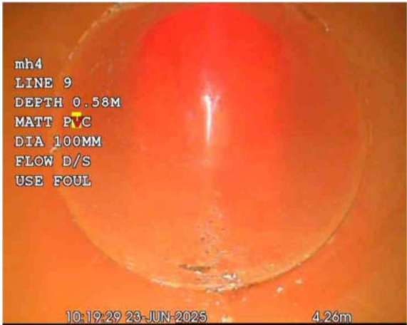
L9X_6a8c22e5-1168-48a0-a32d-5cf0c5b7625a_20250701_165858_809.jpg, 00:00:17, 4.26 m Line deviates up
