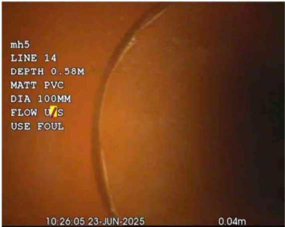
L14X_350b519f-60d0-4551-aa9e-b8f7cb8791cb_20250701_1 65941_811.jpg, 00:00:02, 0.04 m Line deviates right
