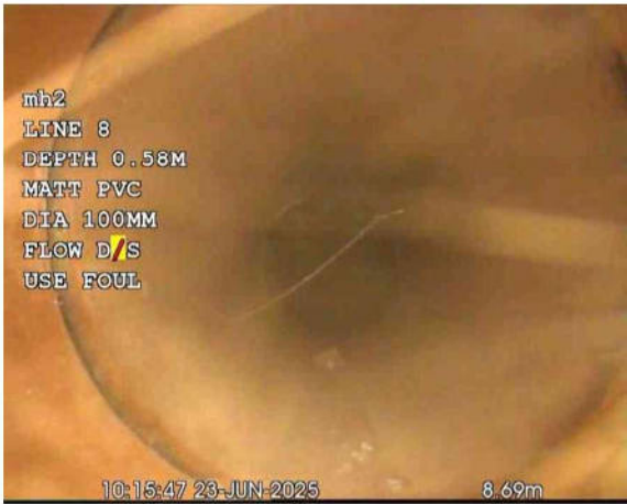
MH 2X_99ede1bb-544a-4a8d-a940-239d07540689_20250701_16 5825_903.jpg, 00:00:37, 8.69 m Pipe size changes, new size(s), 150mm high
