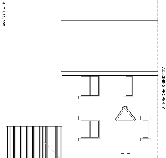
Existing Front Elevation (1:100)
