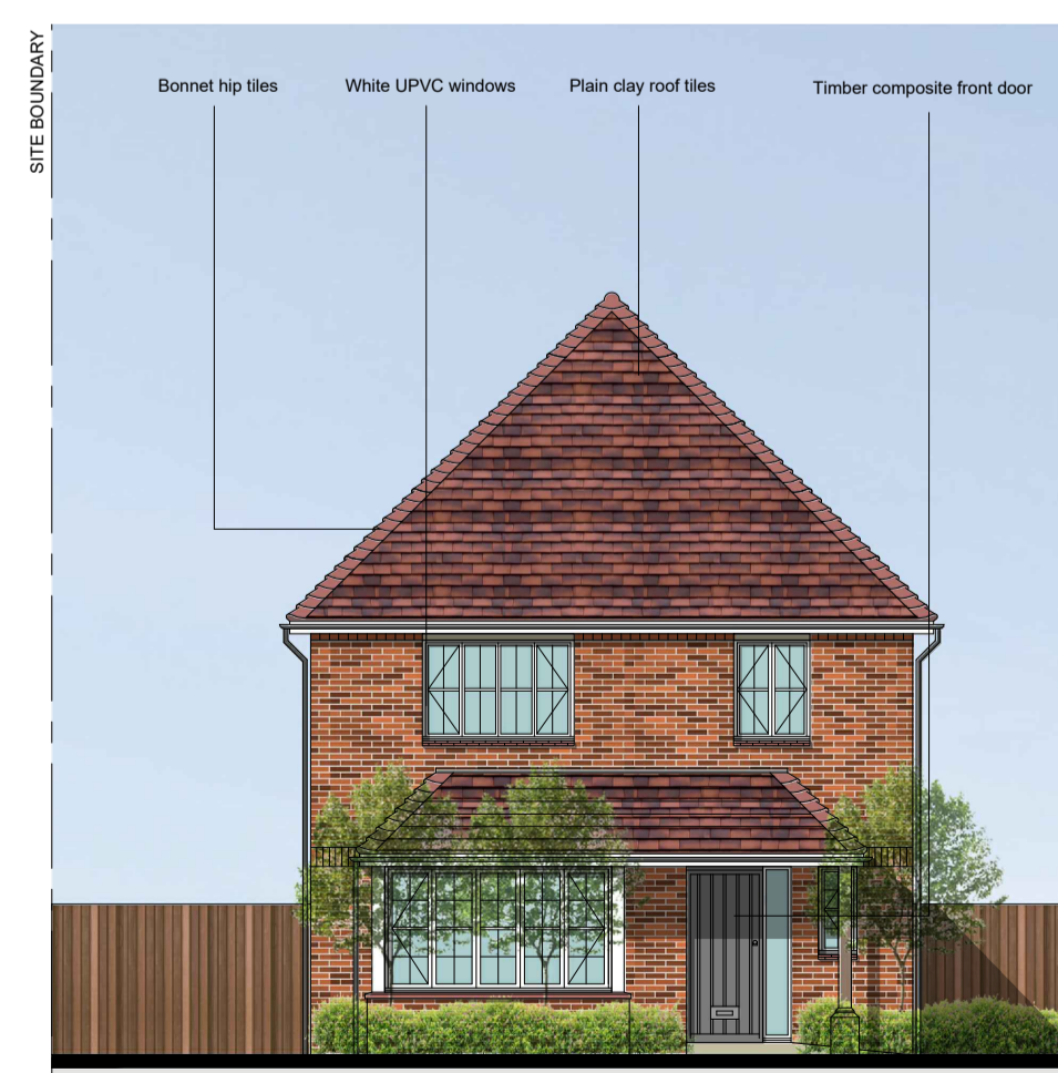
Front (East) Elevation
