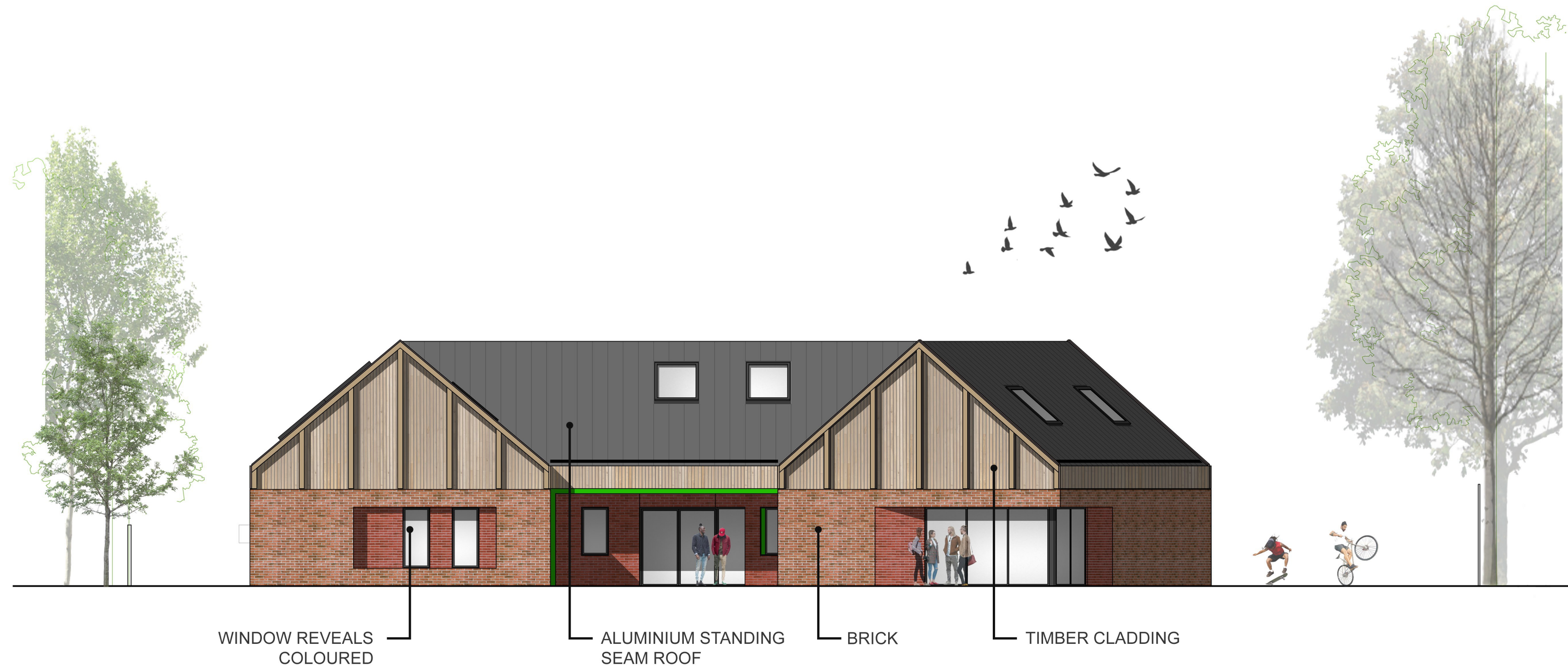
FRONT ELEVATION [NORTH] 1:100
