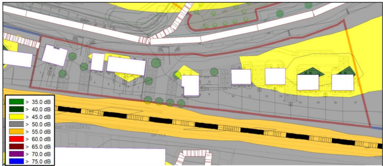
Figure 5.2: Noise Modelling Results - Grid at 4.0m high (night-time)
