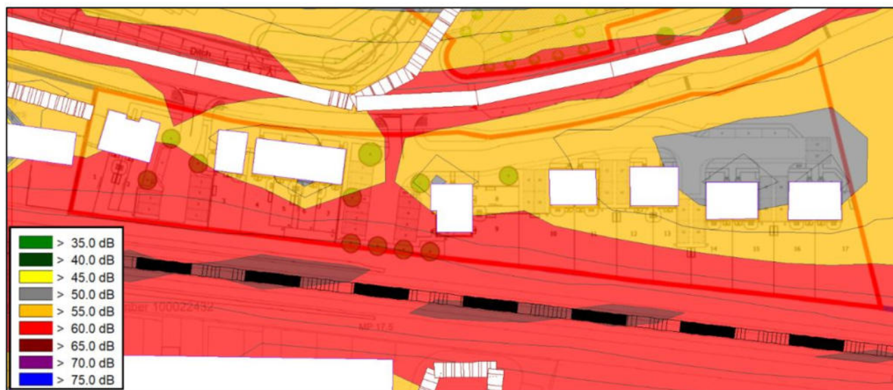
Figure 5.1: Noise Modelling Results - Grid at 4.0m high (daytime)
