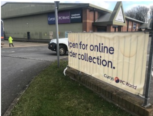
Figure 5: Currys / PC Works banners restricts intervisibility between traffic and pedestrians / cyclists.
