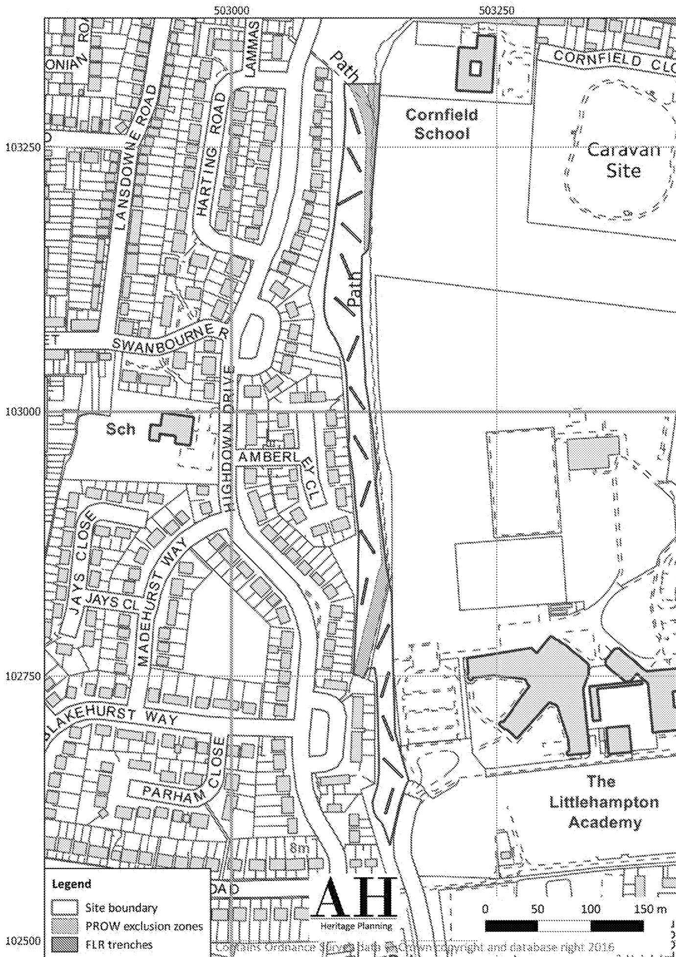
Fig. 2 Trench location plan (Fitzalan Link road - south)
