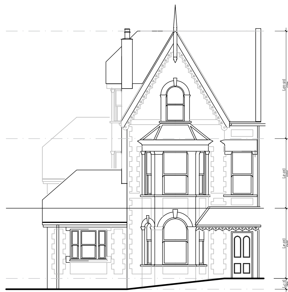
Existing Elevation - South 1:100
