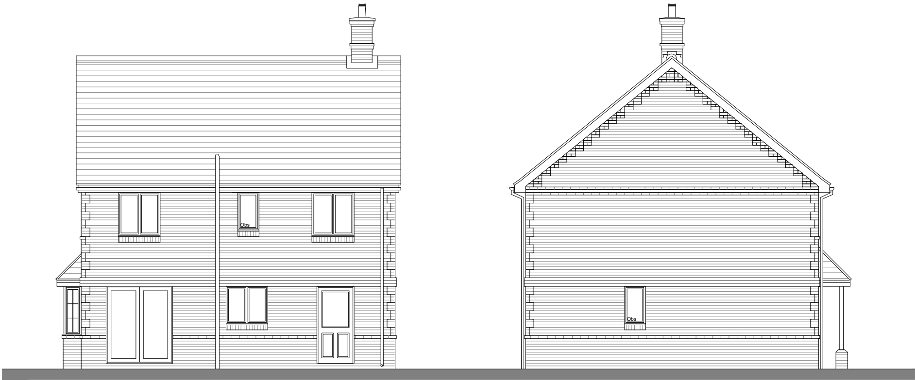
Rear Elevation Obs - Obscured Glazing
