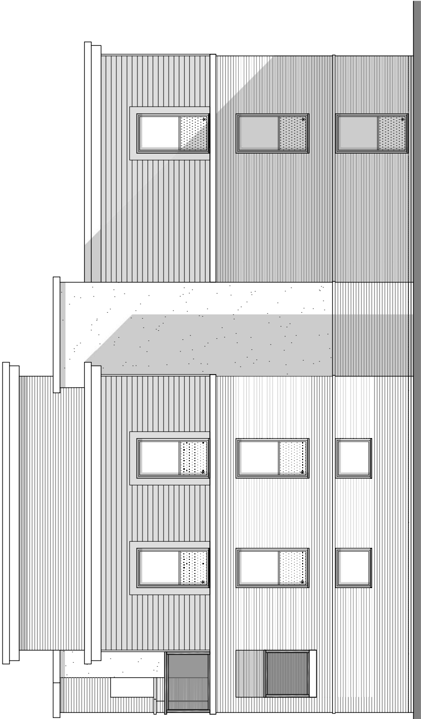
Side Elevation ** - False Panel * - Obscured Glazing
