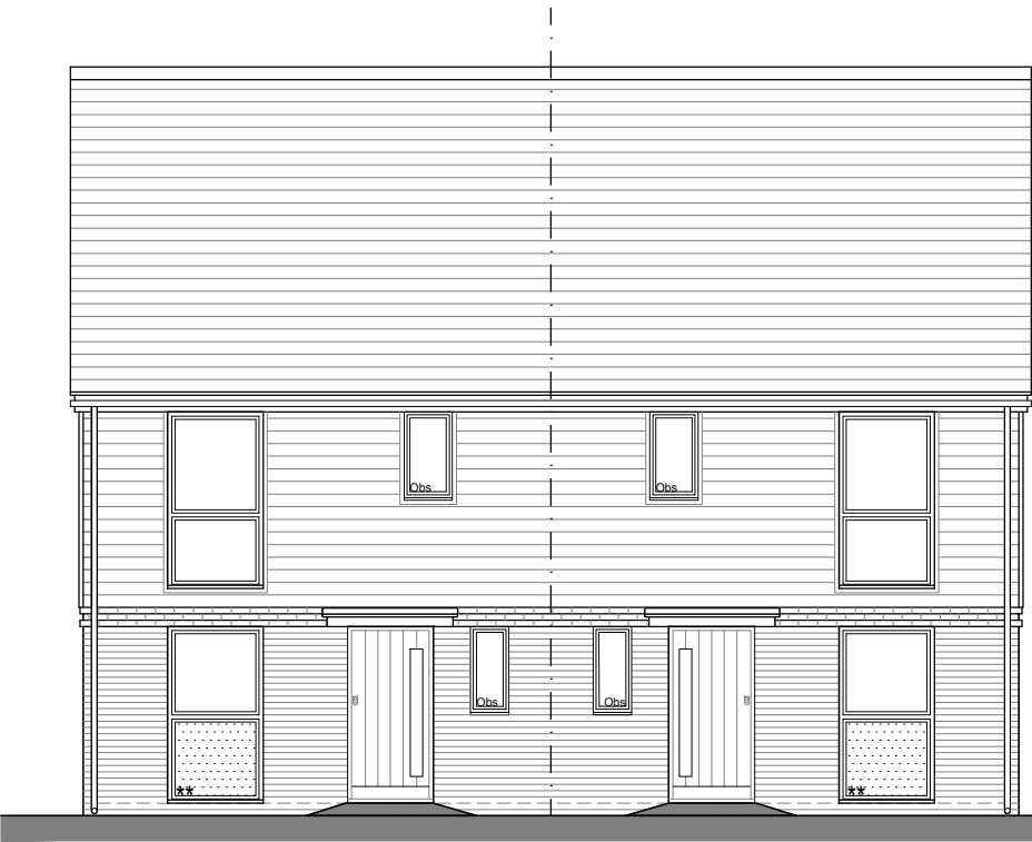
Front Elevation Obs - Obscured Glazing **= False Panel
