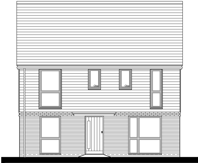
Front Elevation *Obs - Obscured Glass
