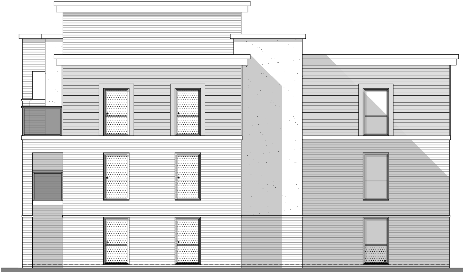
Side Elevation **- False Panel * - Obscured Glazing
