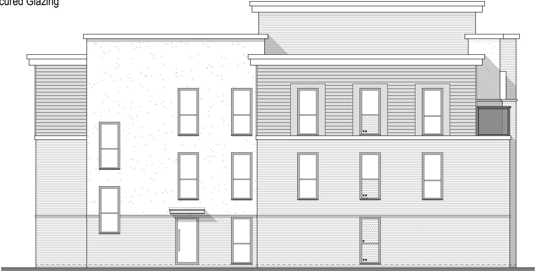
Rear Elevation **- False Panel * - Obscured Glazing
