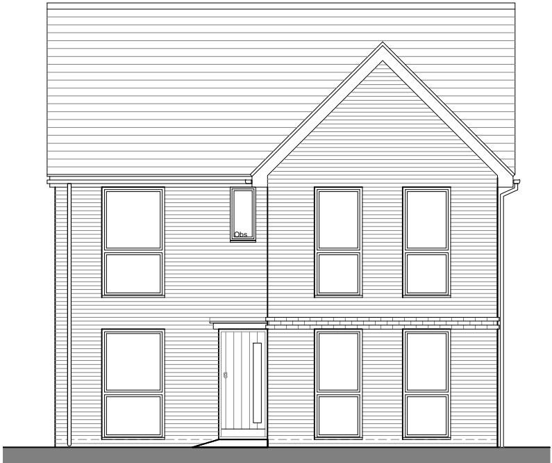
Front Elevation Obs - Obscured Glazing
