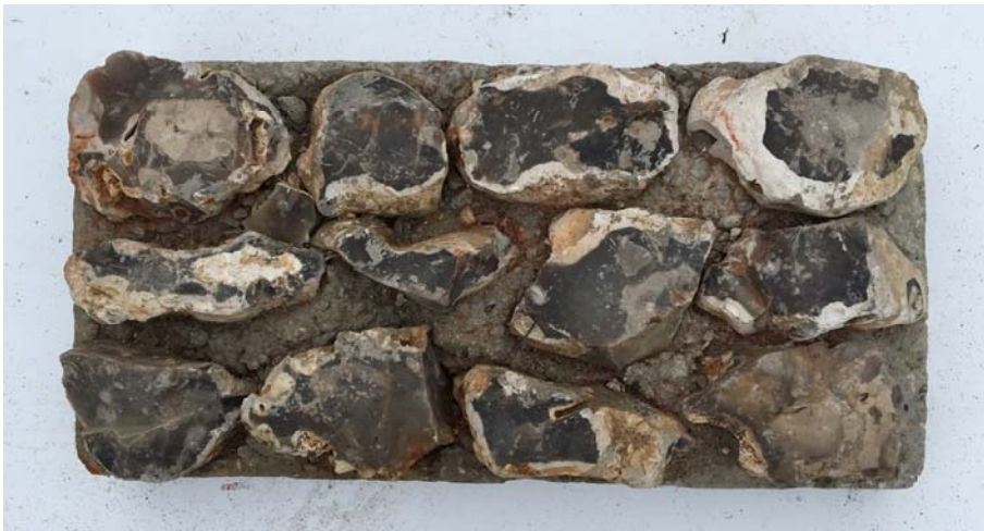
Flint Block (prior to pointing)
