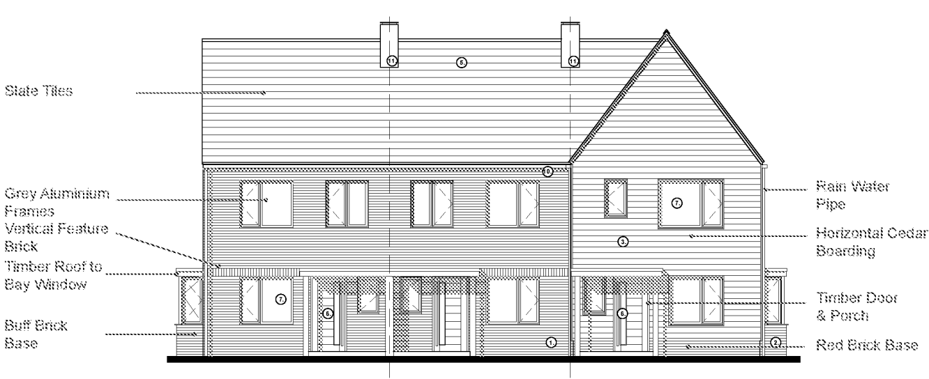
Plots 1-3 Front Elevation - 2 & 3 Bedroom Semi-Detached & Terraced House
