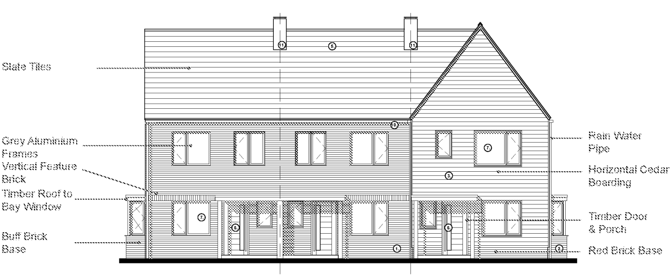
Plots 1-3 Front Elevation - 2 & 3 Bedroom Semi-Detached & Terraced House
