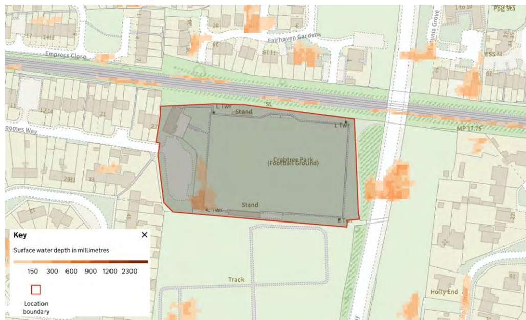
Figure 4.6 Long Term Risk (Surface Water / 1 in 100 year – 2061 to 2125) Source: GOV.UK website – 09/06/2026
