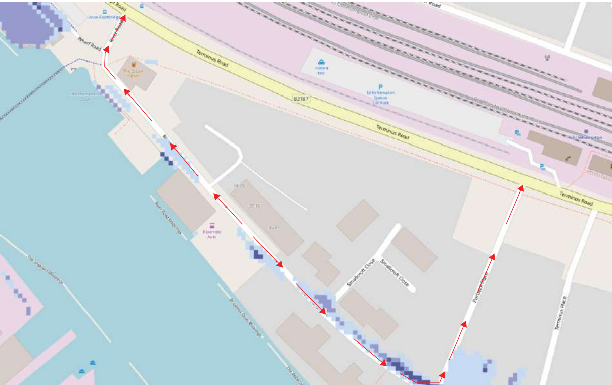
Figure 6.13 Potential Site Egresses During Flood Events
