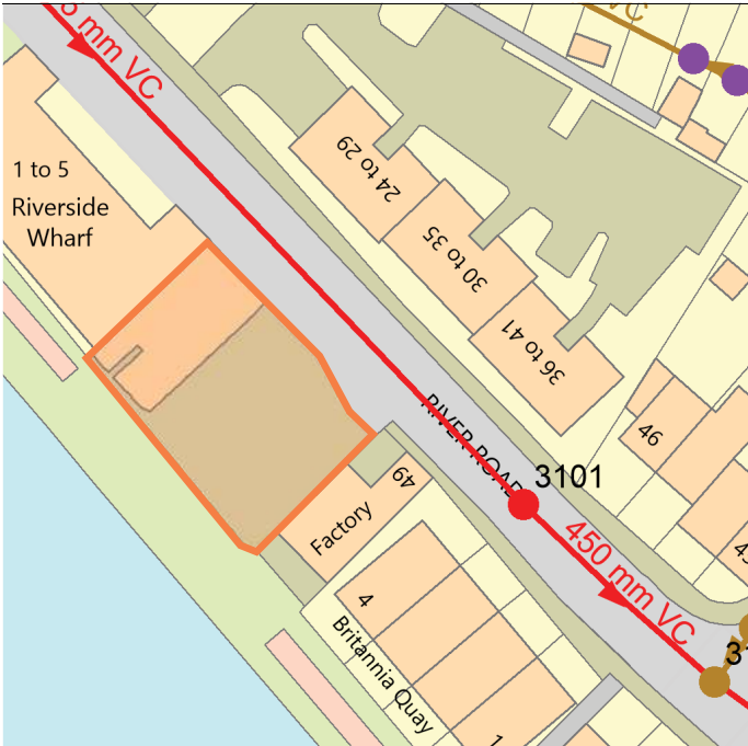
Figure 6.5 Thames Water Asset Record - Sewers
