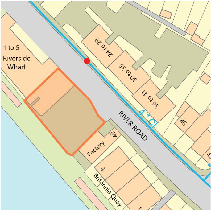
Figure 6.6 Thames Water Asset Record - Water Mains
