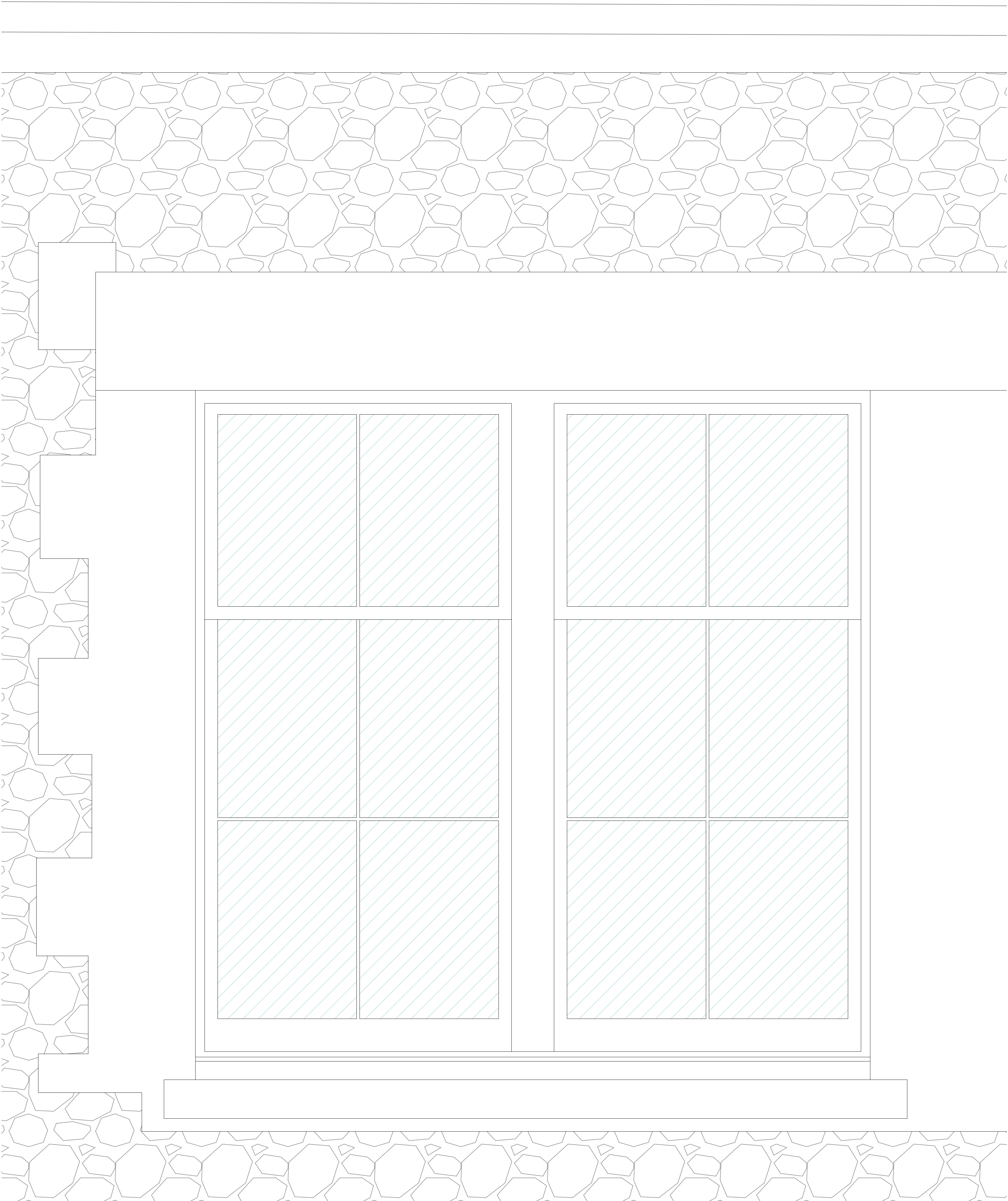
WT05 SASH REPLACEMENT SASH WINDOW ELEVATION - 1:5@A0
