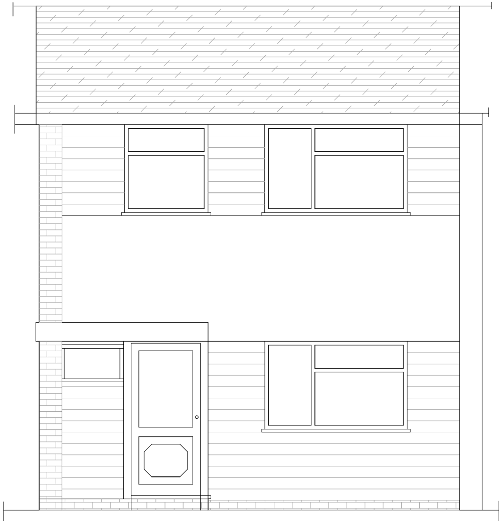
EXISTING SOUTH ELEVATION
