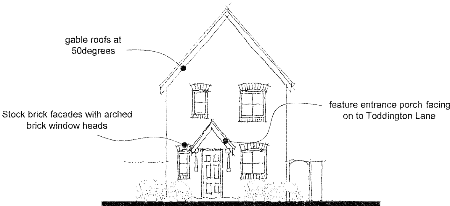
Front Elevation (North)
