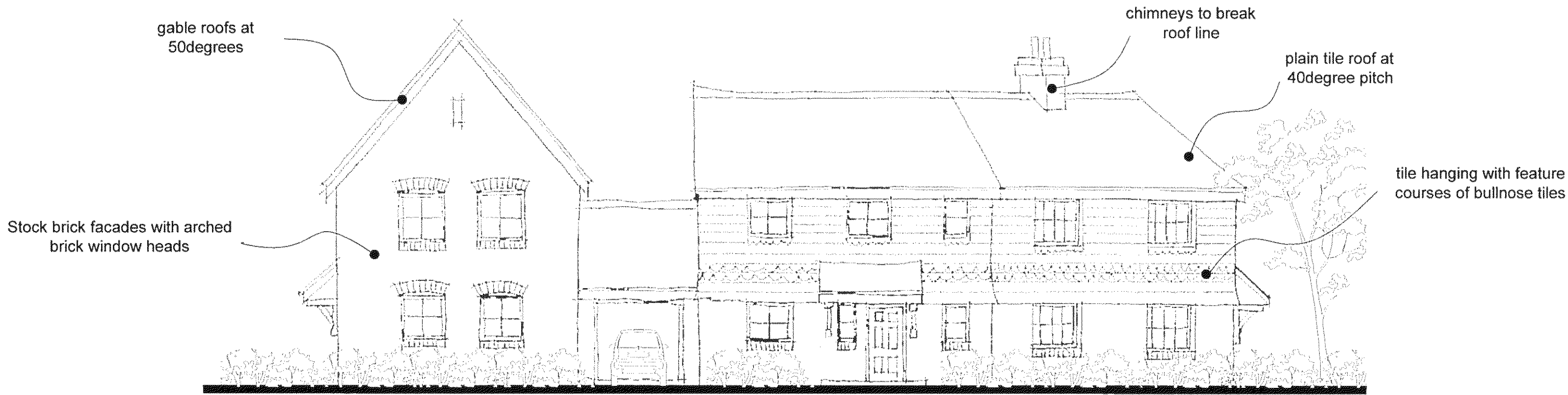
Front Elevation (West)
