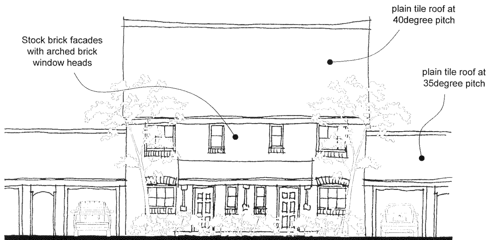
Front Elevation (West)
