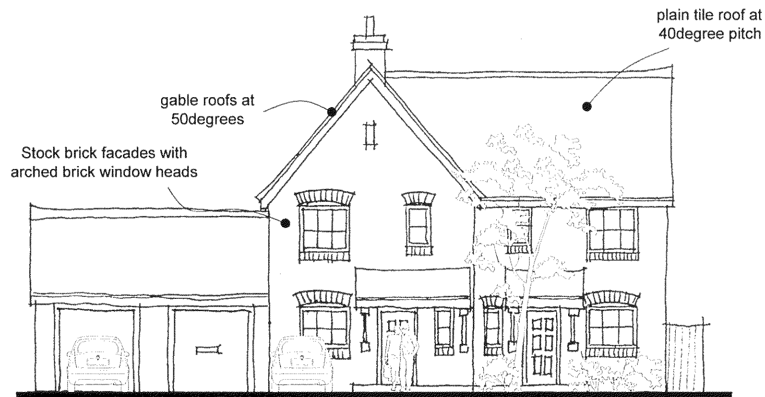
Front Elevation (North)
