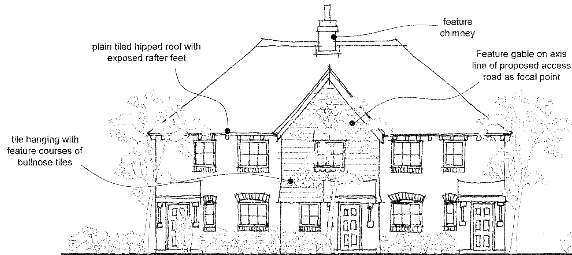
Front Elevation (North)
