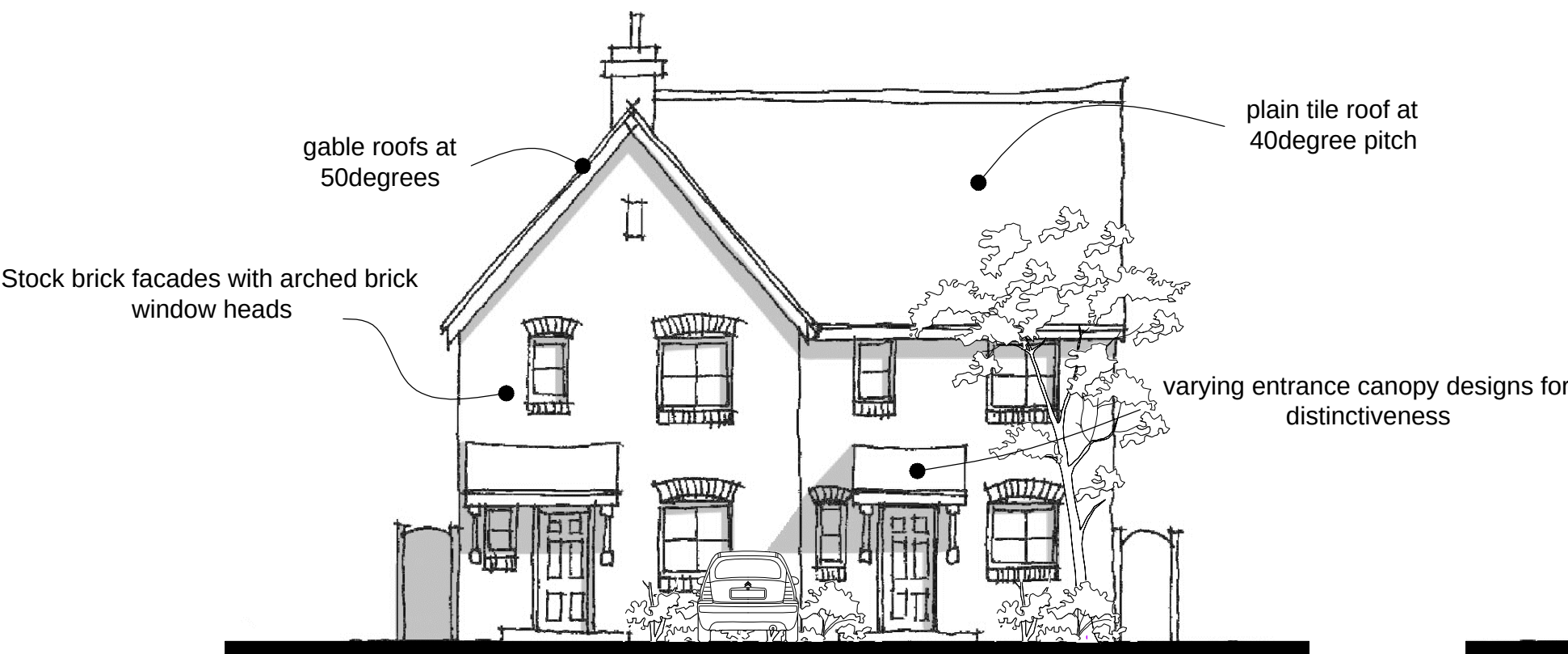
Front Elevation (North)
