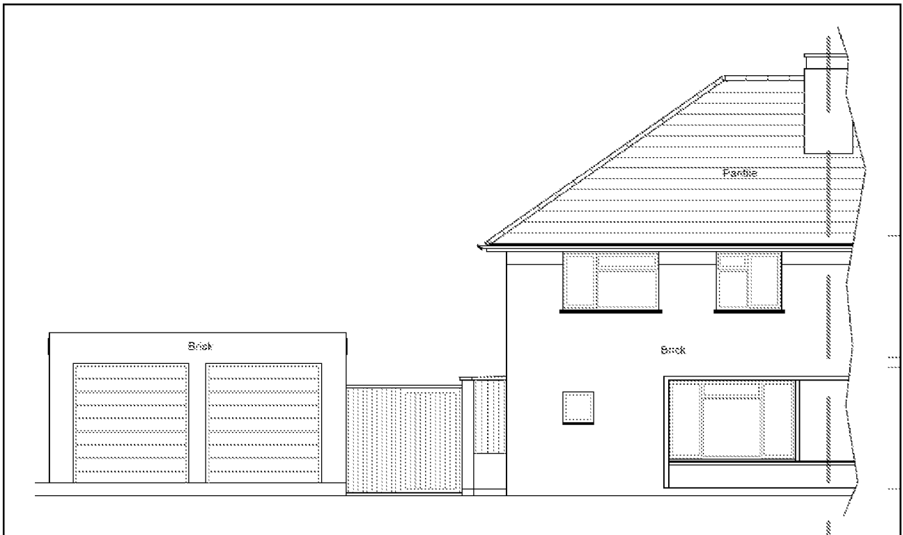
Existing front elevation
