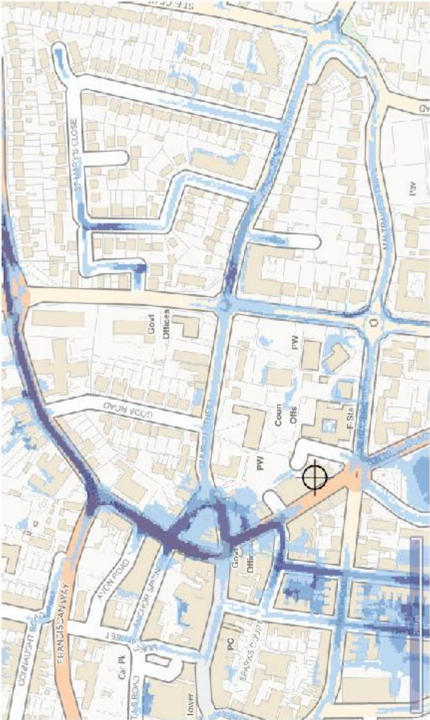
Extent of flooding from surface water
