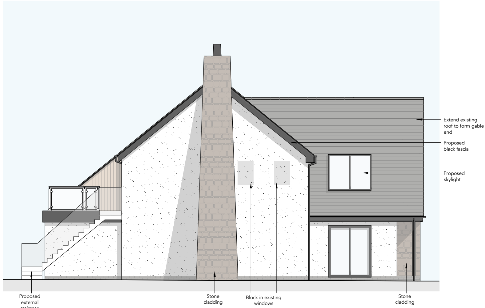
East Elevation (Side)
