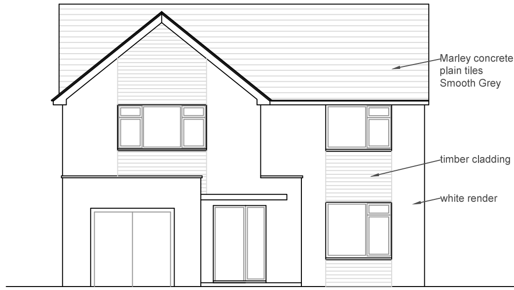
Front Elevation (west)
