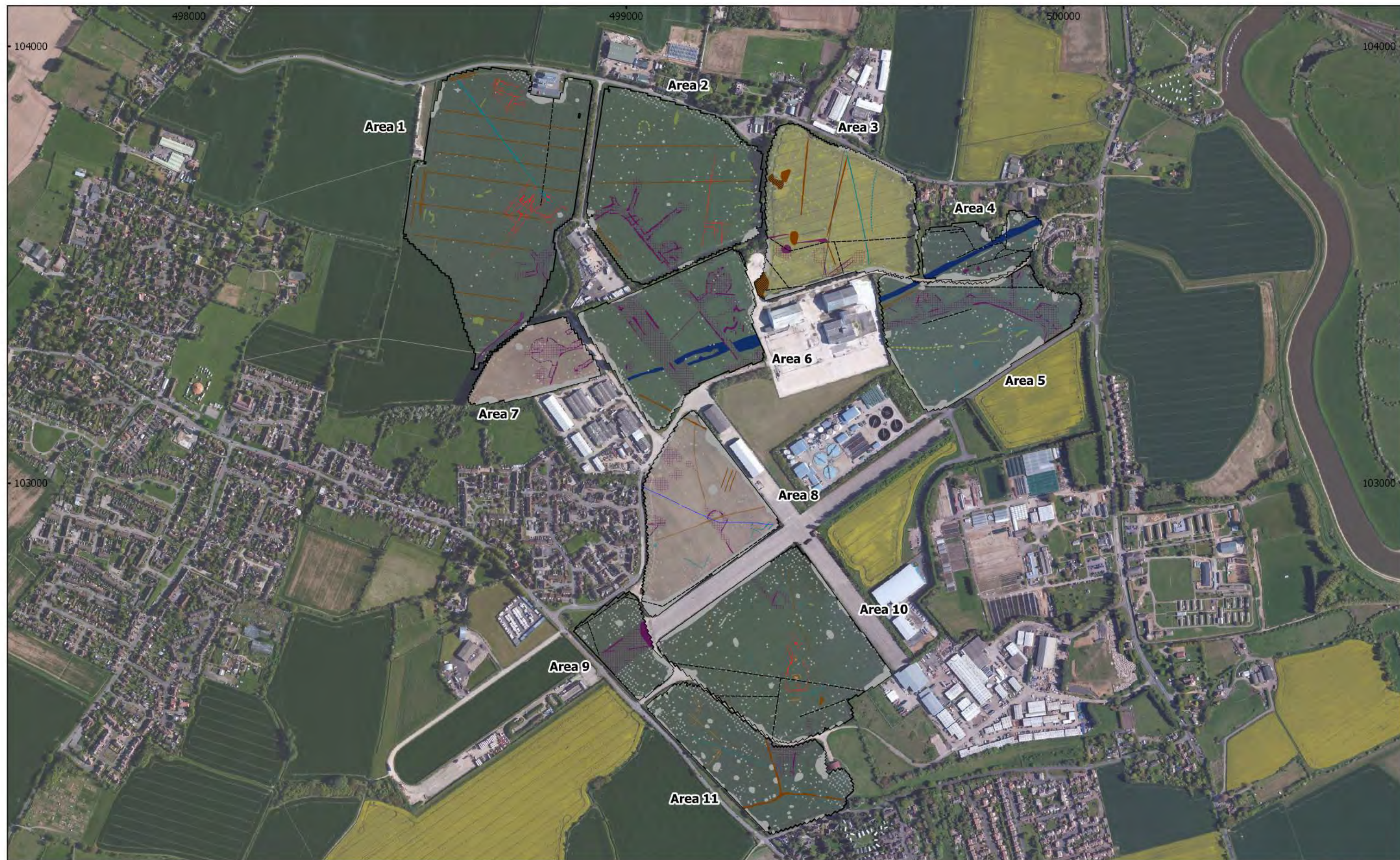
MSSU354 - Ford Airfield, West Sussex Figure 5 - Magnetic Interpretation Over Satellite Imagery Overview 1:8,000 @ A3 Copyright Magnitude Surveys Ltd 2018 Contains Bing Satellite data 2018
