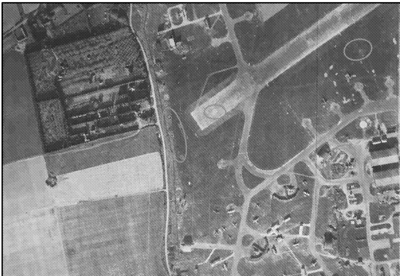
Figure 2. Showing post war bomb damage. Craters are visible and have been circled in red.
